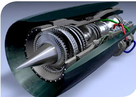
Figura 1. Turborreactor.
